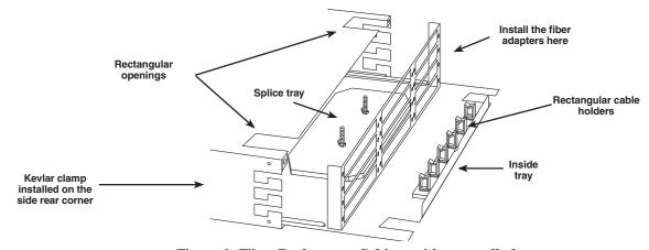
Figure 1. Fiber Rackmount Cabinet with tray pulled out.
