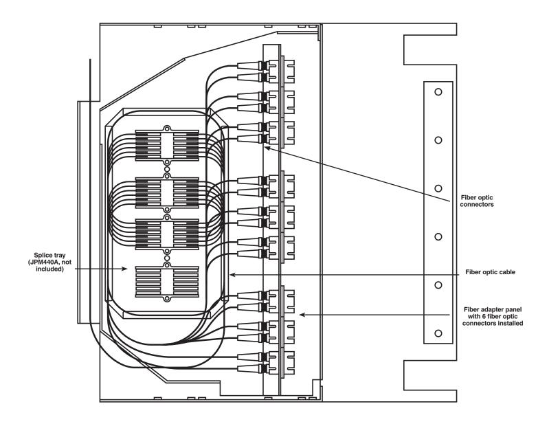
Figure 2. The JPM406A-R5 with three fiber adapter panels visible (up to nine more can be stacked beneath the visible ones, for a total of 12 adapter panels).
