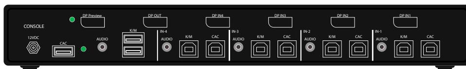
Figure 1-2: KVS4-8004VPX Rear panel
