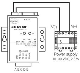
Figure 4.2 Terminal Identification
