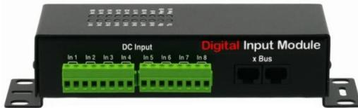
Digital Input Modules with 16 inputs for dry contacts (door contacts, smoke and water detectors...) can be attached to the Power Switch Master to monitor environmental conditions.
