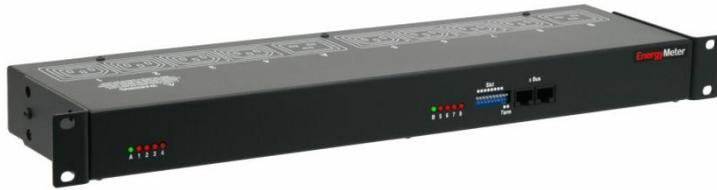
EnergyMeters can be attached to the Power Switch Master to monitor the energy consumption (kWh) and the current consumption (Amp RMS) of eight electrical devices (PC, server, light, printer...) and trigger actions if predefined limits are exceeded. The EnergyMeter is also able to monitor the Input voltage of both 16 Amps power inputs.
